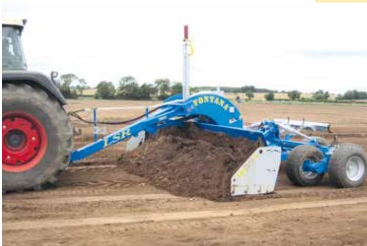
Hydraulic modular automatic levellers preset for zero or double slope laser system with single or double receiving system, slope sensor and GPS.
