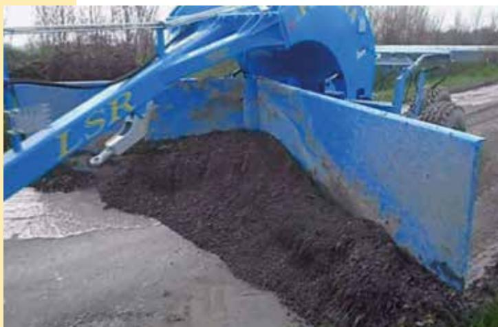
Towed totally hydraulic modular automatic **LEVELLERS** preset for laser system with horizontal plain, simple or double slopes, with proportional receiving system, slope sensors and GPS system.
